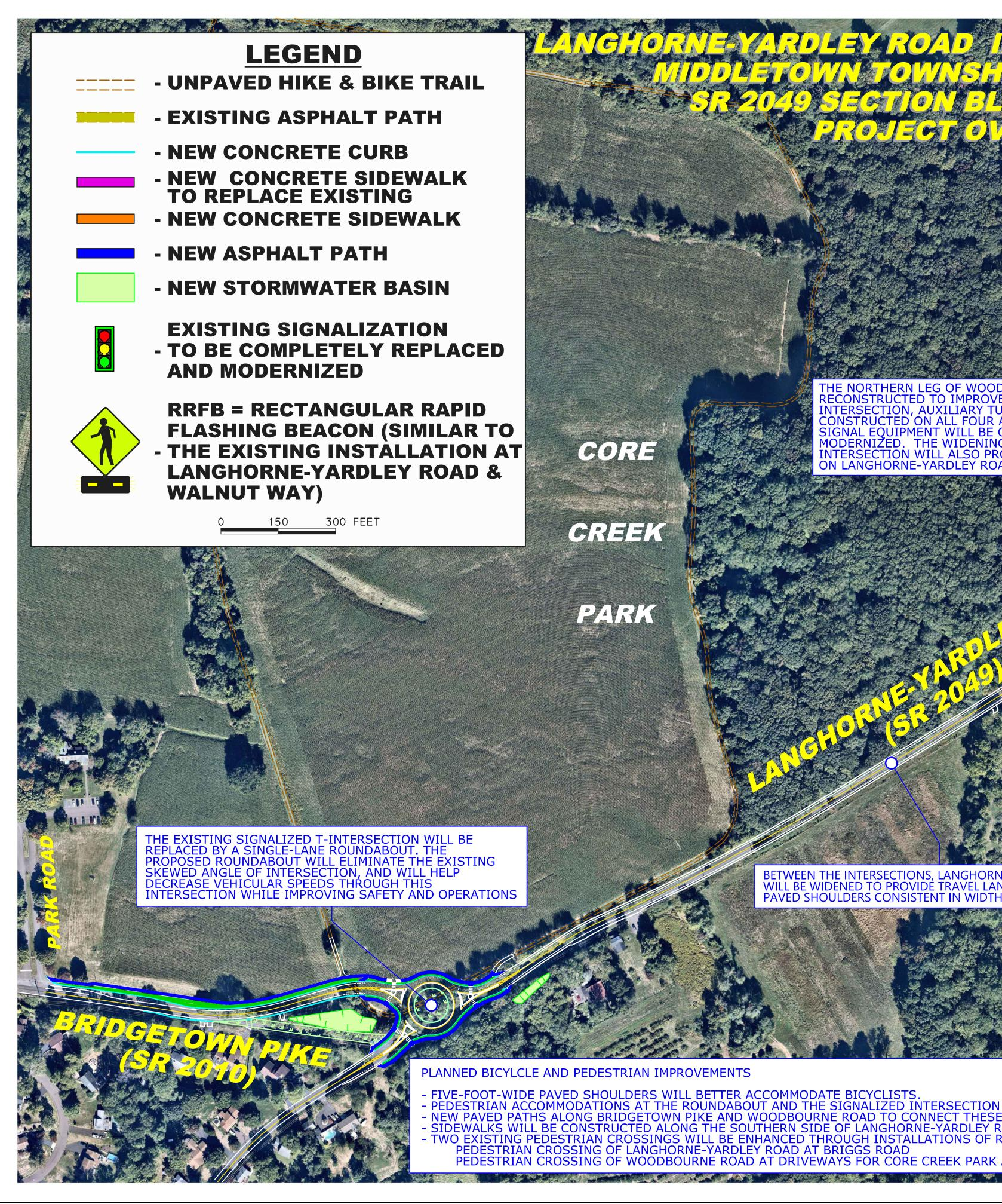
ECONSTRUCTED TO IMPROVE THE ALIGNMENT AT THE ITERSECTION, AUXILIARY TURN LANES WILL BE ONSTRUCTED ON ALL FOUR APPROACHES, AND THE TRAFFI GNAL EQUIPMENT WILL BE COMPLETELY REPLACED AND MODERNIZED. THE WIDENING OF THE EASTERN LEG OF THE INTERSECTION WILL ALSO PROVIDE FOR A LEFT TURN LAN
